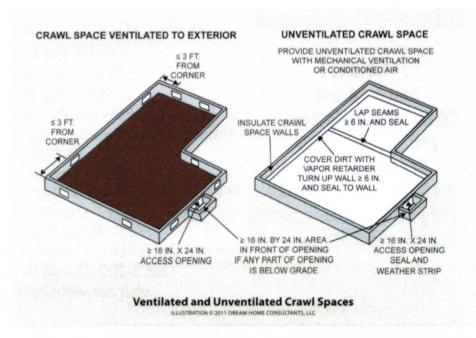
unintended pressure differences between the crawl space and the home. The airflow rate should be maintained near the recommended rate, again because of the potential for unintended pressure difference between the crawl space and the home. The airflow rate is a case where more airflow isn't necessarily better.
